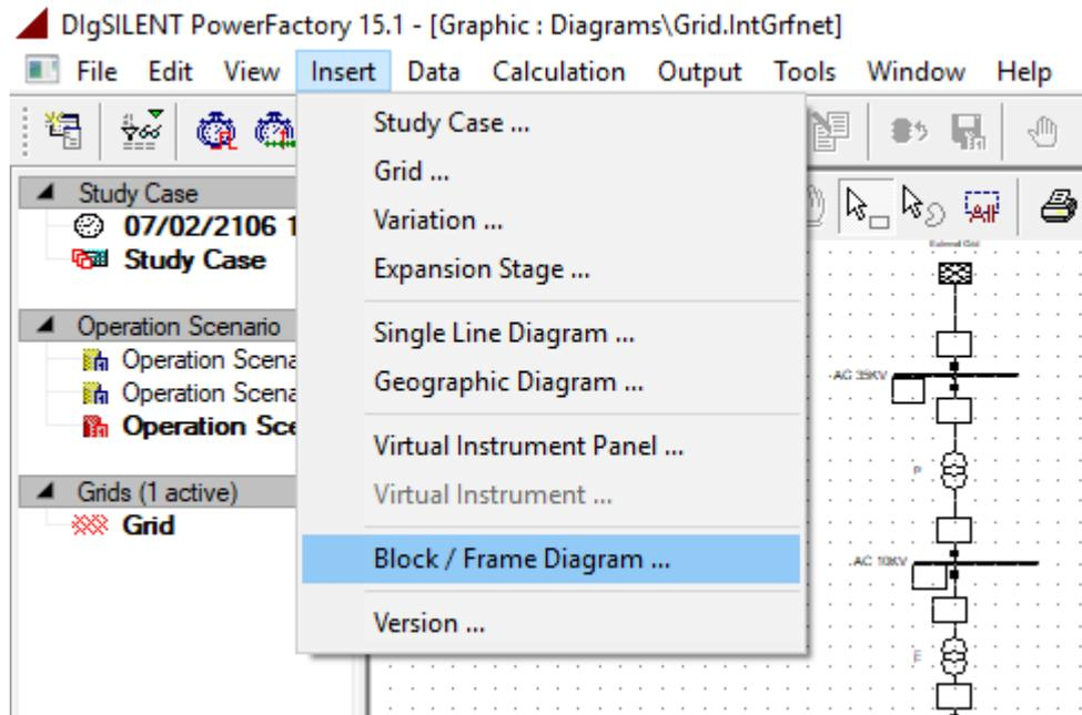
**Fig. 6 Insertion of Block/Frame Diagram**
