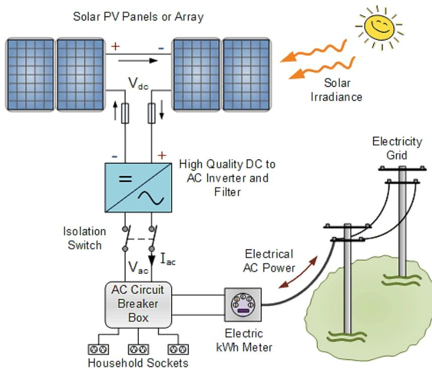
**Fig.1 The concept of the Grid-connected PV system**
