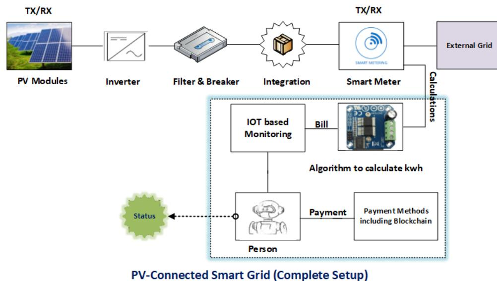
**Fig. 17 Infrastructure of Smart Meter Integrated in Smart Grid**
