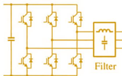
**Fig. 8 Topology of the Solar Inverter**
