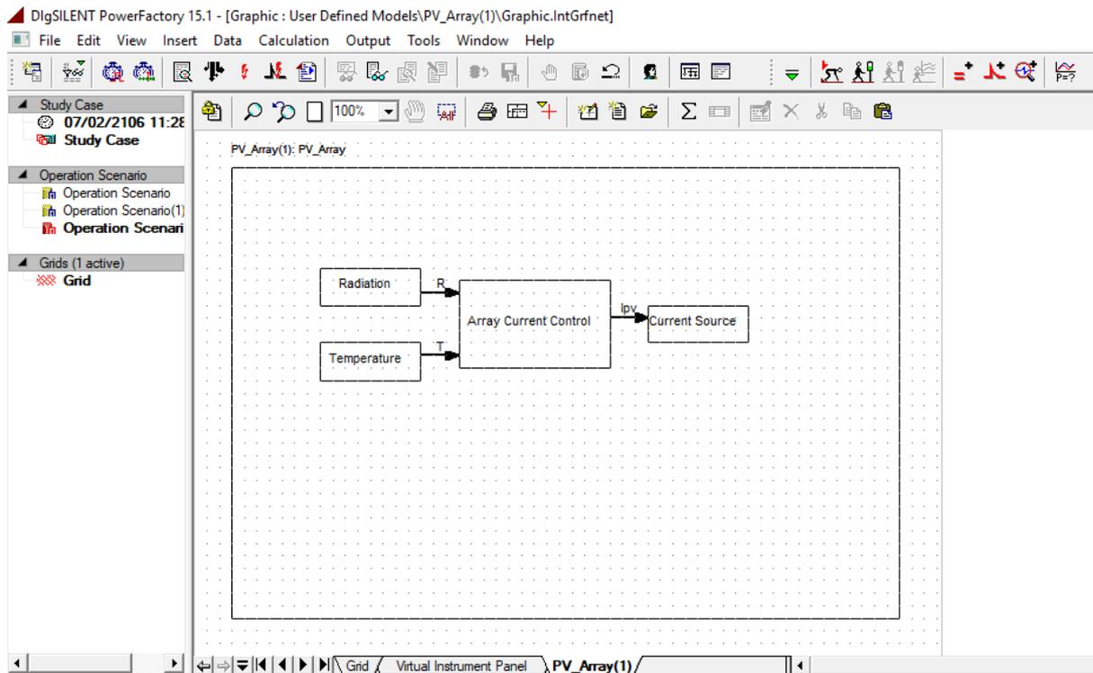
**Fig. 7 Modelling of the PV Array**
