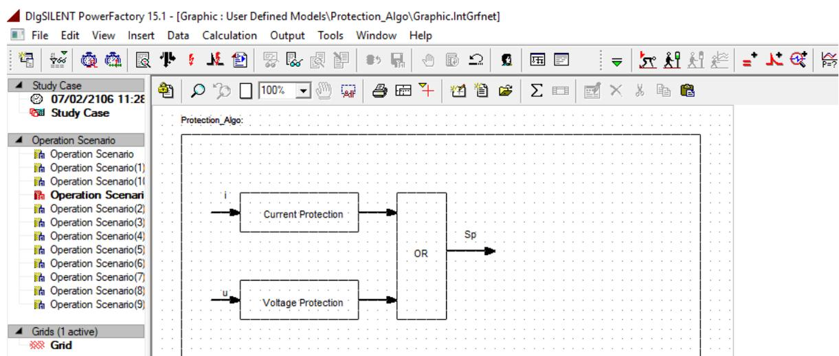
**Fig. 15 Modelling of the protection algorithm in the DigSilent power factory**
